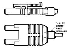
The duplex latching connector is designed for rugged applications requiring greater retention force than the nonlatching duplex connector. When inserting the duplex latching connector into a module, the connector latch mechanism should be aligned with the top surface of the dual combination of horizontal or vertical Versatile Link components. The duplex latching connector is available in gray (HFBR-4516) or black (HFBR-4516B).
