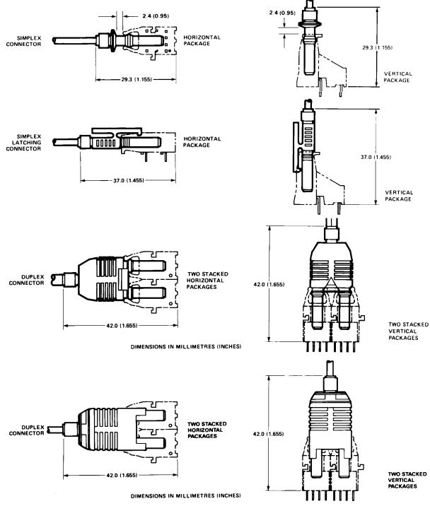
Bulkhead Feedthrough or Panel Mounting for HFBR-4501/4511/4501B Simplex Connectors
