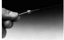
Insert the stripped cable through the guide hole of the fiber stripper tool, inserting the crimp ring until it is fully seated in the guide tube. Holding the unstripped cable securely, squeeze the handles of the fiber stripper to cut the fiber buffer and pull straight to slightly separate the buffer.
