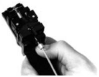
Carefully insert the ferrule into the slot on the diamond cleave tool until the ferrule rests securely in the cleave tool connector adapter.
