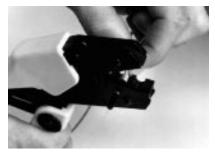
Slide the ferrule onto the fiber and into the crimp ring, carefully aligning the ferrule fully within the crimp ring. The fiber should protrude at least 35 mm (1.4 in) through the end of the ferrule. Selecting the large hole on the crimp tool (rear die nest), crimp the ring to the ferrule by fully squeezing the crimp tool handles together and releasing.
