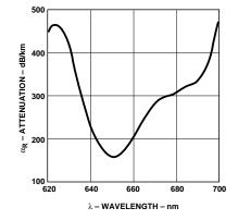
Figure 1. Typical POF Attenuation vs. Wavelength.
