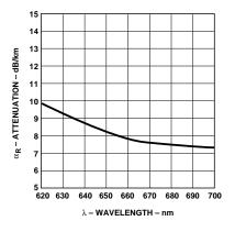
Figure 1. Typical HCS Attenuation vs. Wavelength.
