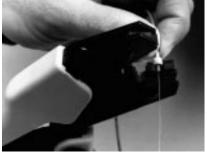
Place the crimp ring over the end of the cable and rest the larger end against the unstripped cable jacket. Selecting the smaller crimp hole (front die nest), align the crimp ring in the crimp tool jaws and fully squeeze the tool handles together and release. This crimps the crimp ring to the fiber buffer.
