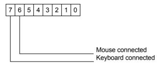
The *StatusIndicator* can be used to check whether a keyboard or a mouse is connected to a PD 5020 VGA Controller.
