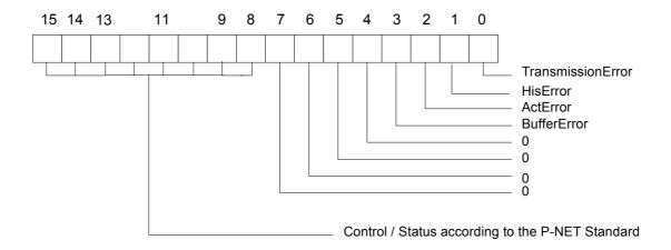
The format for the error code in PD 5000 is different from the error code that is used in PD 4000. A procedure, called *ConvertErrorCode* that is able to convert from the PD 5000 error code format to the PD 4000 error code format is available in the PD5000SP.INC file.
