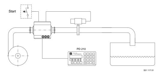
The PD 340 flow transmitter has a built-in batch control function, and can therefore easily be used to control the dosing of a specified volume. The requested volume is keyed into "SETPOINT" on the PD 210. Input 1 on PD 340 is used to start the batch control. Output 2 controls the dosing valve or pump. The Volume 2 counter shows the dosed volume. When the batch control function is used, the built-in flow regulator cannot be used.
