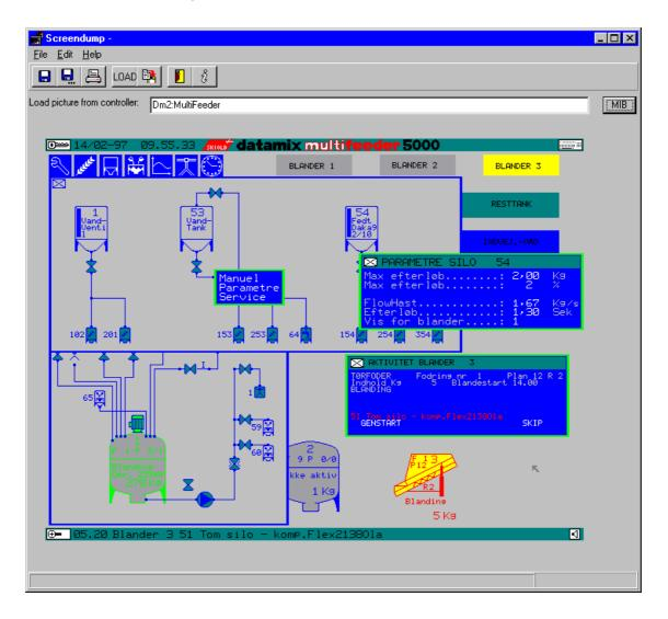
*Screen Dump* can be started from the MIBOCX, using the right mouse button menu, when a node of the following controller type is selected: PD3010, PD4000 or PD5010, PD5015 or PD5020. These form one of the Object Types - 3000, 4000 or 5000.
