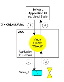
The valve is closed (set to OFF) using the following code: Object1.Value = OFF
