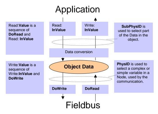
A Read of a variable within a node into an application is divided into two steps. First, the content of the variable is loaded into the Object Data. The next step is to convert the received data, and then transfer the converted data to the application. A similar situation occurs to Write, except that the first step is to convert data sent from the application, and then to store the converted data in Object Data.
