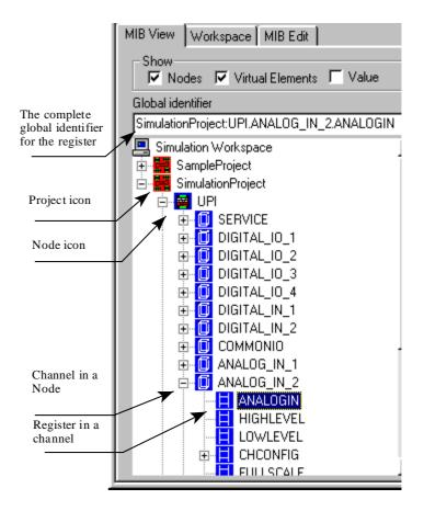
A **Node** within the Project description (the MIB), is defined as a module or a unit within the physical plant (e.g. a PD3221- Universal Process Interface, UPI). Each Node is represented by a *Node icon* in the MIBOCX.
