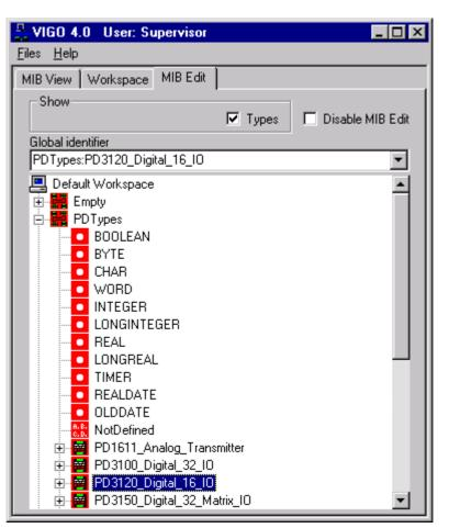
LongReal, Timer, RealDate and OldDate. The *Array Type Element* also belongs to this group, and is represented by a red *Array type Icon*. The properties of an Array type element holds information about the type structure of the Array elements, as well as the minimum and maximum index for the Array. A string is a special form of an Array (consisting of an array of characters) and is represented by a red *String type Icon*.
