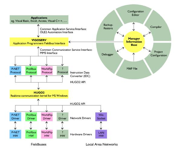
All this makes VIGO an open system, which can always be expanded for inclusion of new network connections to physical objects, and new tools for configuration. It is open, in the sense that anyone can provide a network or tool implementation, and anyone can develop an application that uses the communication functions offered by VIGO.
