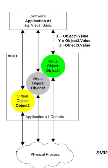
(Read valve state) Y = Object2.Value (Read temperature) Z = Object3.Value
